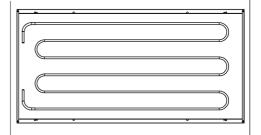
CBL smooth: max. 83°C / max. 6 bar CBL perforated: max. 50°C / max. 6 bar ALL smooth/perforated: max. 83°C / max. 6 bar PAM smooth/perforated: max. 50°C / max. 6 bar
